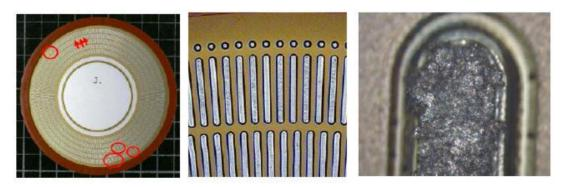
Figure 10: Cathode side of wafer, middle picture shows contact finger arrangement, right picture shows burned contact finger with almost an cathode-anode short
