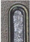
**Figure 12:** Cathode side, contact fingers show very little wear-off.
