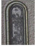
**Figure 12:** Cathode side, contact fingers show very little wear-off and some burned spots, which are uncritical.
