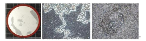
**Figure 9:** Anode side of wafer with partly melted aluminium contact layer. The middle picture is enlarged 45x, right picture 440x
