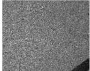
Figure 11: Anode side of wafer shows uncritical small spots in aluminium contact layer.
