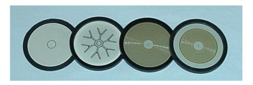
Figure 1. Si-Wafers Ø51 mm for di/dt < 0.1kA/ms, 1kA/ms, 18kA/ms and 15kA/ms. The right one is with a monolithic integrated freewheeling diode.
